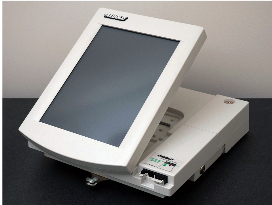
Figure 7.1: The Diebold AccuVote-TS was the most common DRE in the U.S. [26].
