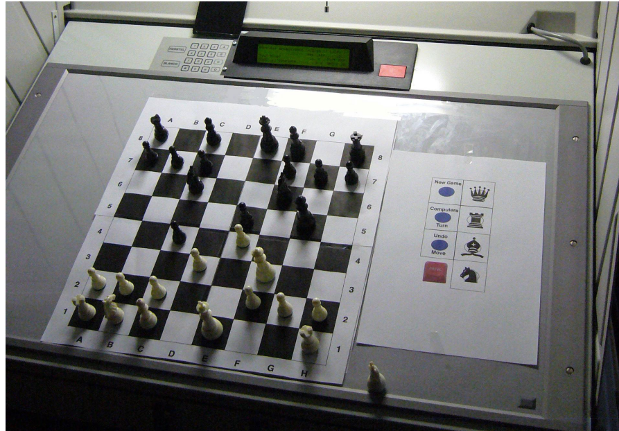
Figure 7.5: Dutch researchers showed that they could quickly replace the firmware ROMs in the Nedap ES3B DRE to tamper with votes ... or make it play chess [28].
