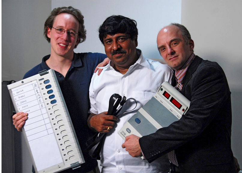
Figure 7.7: Halderman, Prasad, and Gonggrijp studied an Indian DRE provided by an anonymous whistle-blower [81]. The simple embedded system design consists of a ballot unit used by voters ( left ) and a control unit used by poll workers ( right ).
