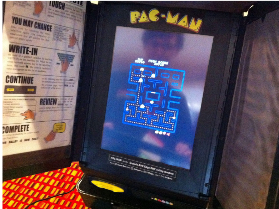
Figure 7.4: Voting researchers converted a surplus Sequoia AVC Edge DRE into a working PAC-MAN machine to show how easily its software could be modified [33].
