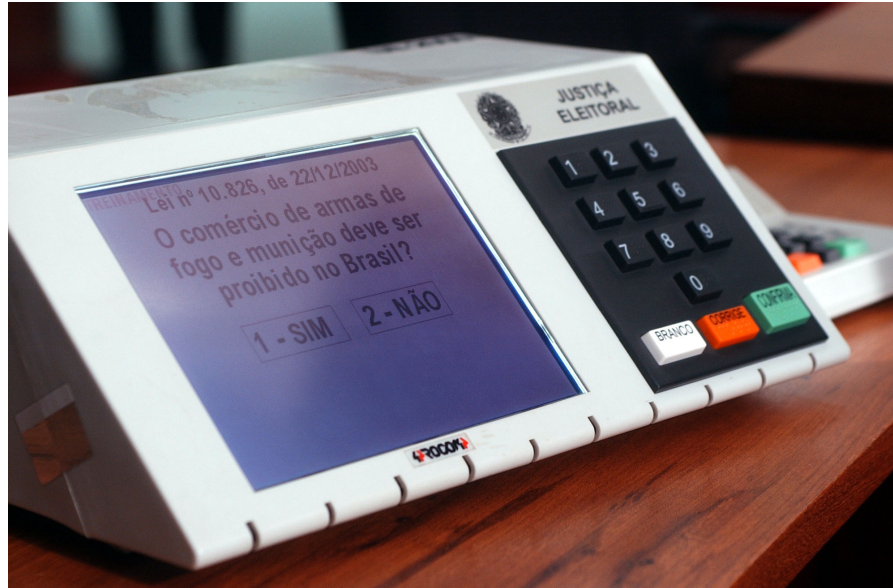
Figure 7.6: Brazil’s DRE voting machines failed to properly shuffle electronic vote records, potentially allowing malicious insiders to deanonymize them.
