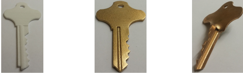
(a) 3D printed nylon plastic Best G key (b) 3D printed brass SC1 key (c) Brass KW1 key, twisted 90 degrees
